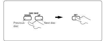
• The disc number can be selected directly by using the numeric keys in place of the **DISC SKIP(DOWN/UP)** keys.
